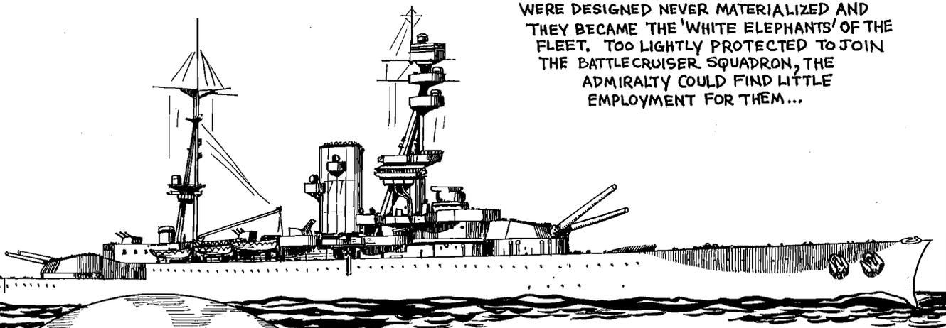
H.M.S. GLORIOUS AND H.M.S. COURAGEOUS AS ORIGINALLY COMPLETED, CARRIED FOUR 15-INCH GUNS AND 18 4-INCH GUNS IN TRIPLE MOUNTS AT 32 KNOTS. COURAGEOUS WAS EMPLOYED FOR A TIME AS A MINELAYER!
