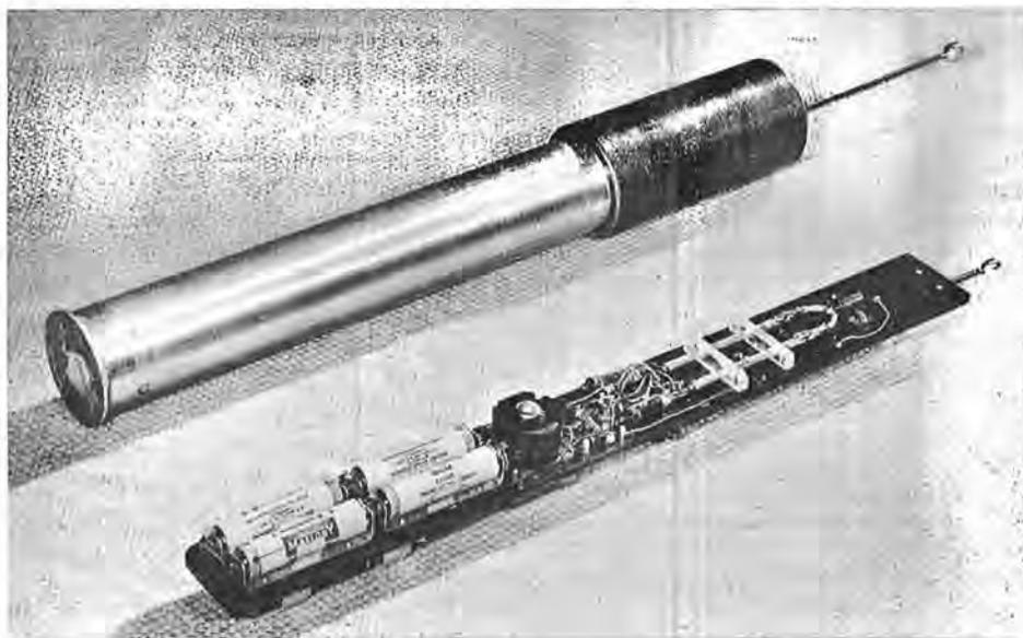
This is the new distress beacon developed by the National Research Council. The compact device weighs only three pounds, is buoyant and its signal has a range of 34 miles. (NRC Photo)
