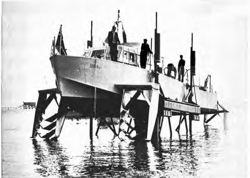
Tests began in 1957 of the Bras d'Or, joint DRB-RCN project to explore possibility of using hydrofoils on smaller RCN craft to enable them to operate at high speed in rough water, particularly for air-sea rescue. The 59-foot craft is being tested by the Naval Research Establishment in Halifax. (DRB Photo)
