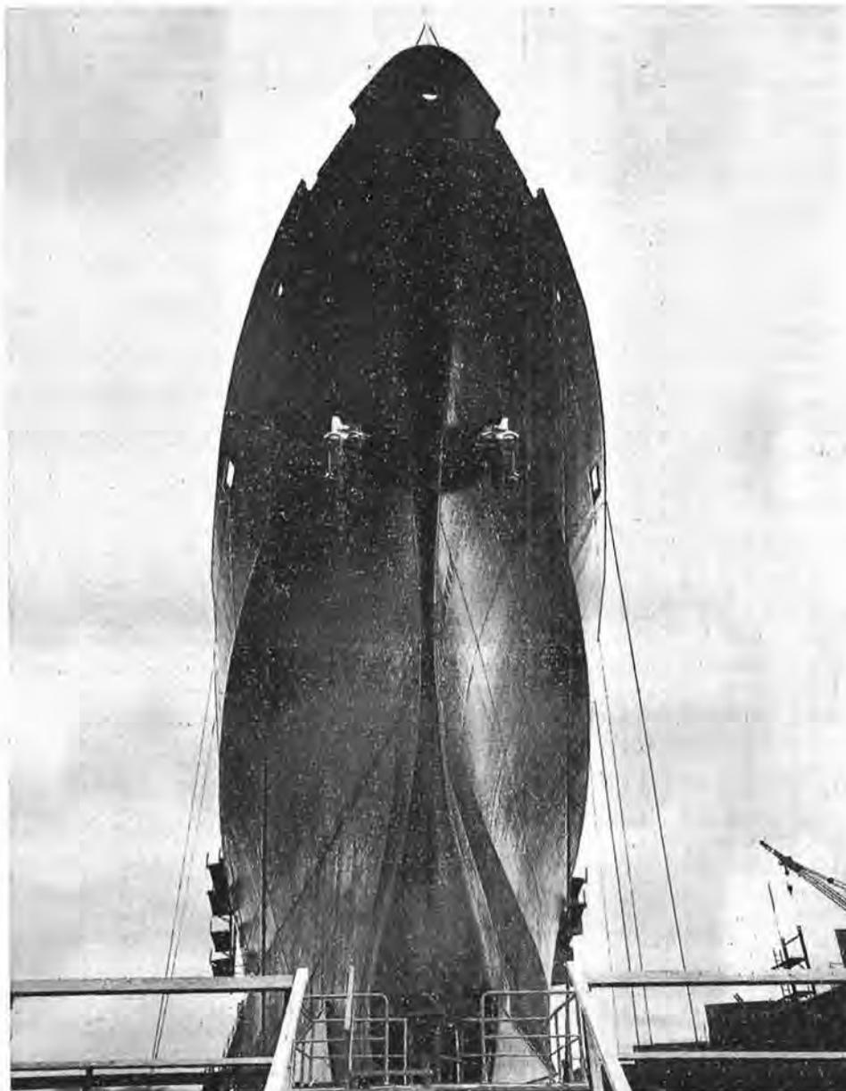
Almost as high as a seven-storey building, the tanker supply ship *Provider* towers above the launching cradle at the Lauzon shipyard where she is being built for the RCN. The actual height is 65½ feet. Her overall length of 551 feet means that, stood on end, she would match the height of a 55-storey building (ML-11175)
