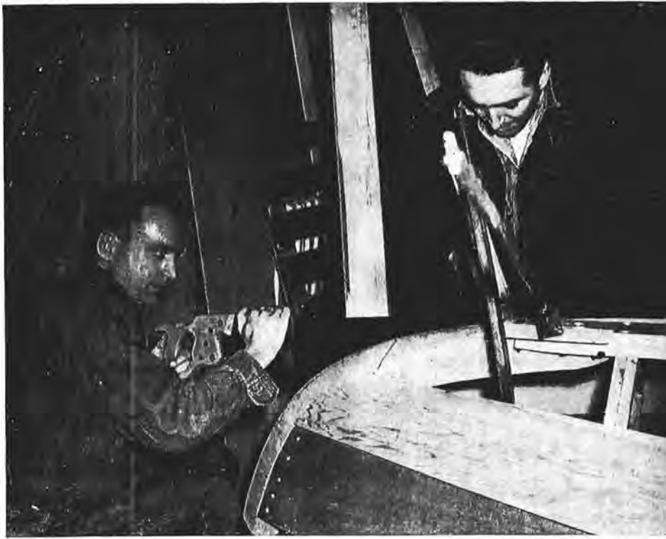
Chief Petty Officers Peter Cox (left) and Bill Peakman set in place the garboard strake of one of the Snipe class yachts being built by the RCN Yacht Club at Esquimalt. Neither had previous experience at boat building before joining the club. (E-11086.)
