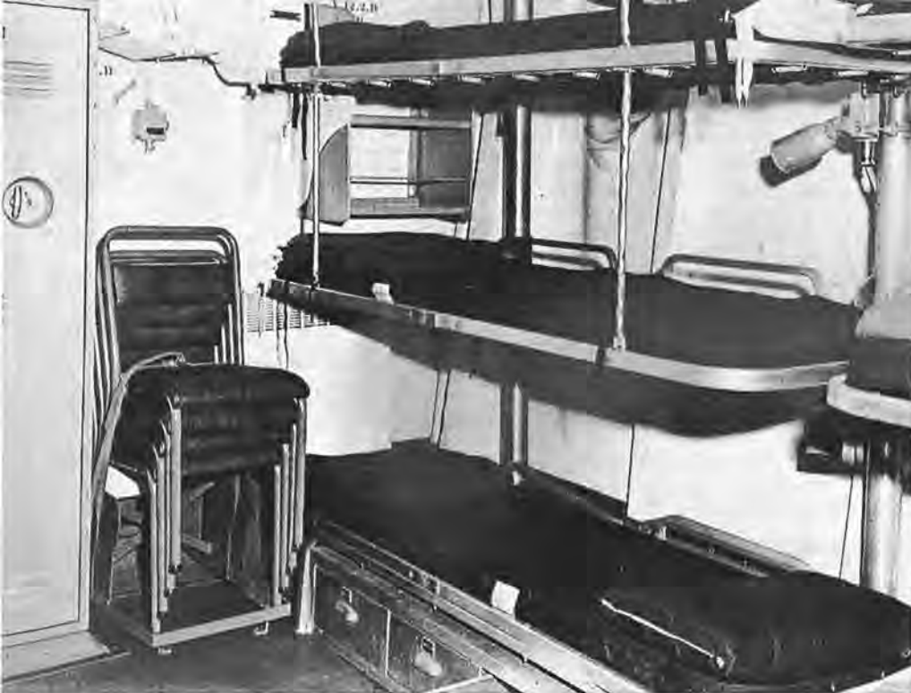
This shows a corner of a Chief and POs' mess. The middle bunk can be lowered to form the back for a settee. Bunks are equipped with individual reading lamps and foam mattresses. Gear is stowed in drawers below bottom bunk and in individual lockers, of which one is shown at the left. Nesting chairs provide additional seating. (ML-1510)
