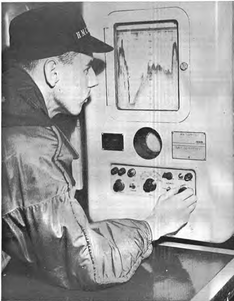
"The Moving Finger writes: and, having writ. Moves on: nor all your piety nor wit Shall lure it back half a line, Nor all your tears wash out a word of it." The "Moving Finger" in this instance is the electric stylus which traced the graph on the Labrador's echo-sounder as the ship ventured into the uncharted waters of Bellot Strait. Eyed closely by Ldg. Sea. Charles Musgrove, the trace shows a sudden plunge from 50 feet—the shallowest depth recorded in the channel—to 600 feet and then up to 100 again, showing that the submarine landscape of the Arctic can be pretty rugged. (LAB-2248)
