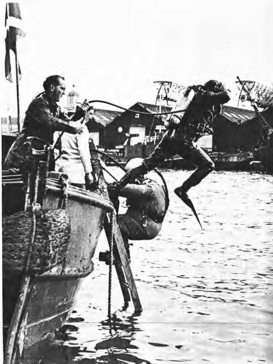
A new lightweight diving suit to replace the cumbersome equipment now used by deep-sea divers is being tested by the Royal Navy. The new suit, shown under test near Portsmouth, embodies many of the features of the frogman type suit and eliminates the heavy metal helmet and lead-weighted boots. (Photo from U.K. Information Office.)
