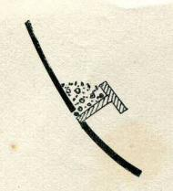
Advantage may sometimes be taken of the ship's framing or stringers to support concrete while it is setting.
