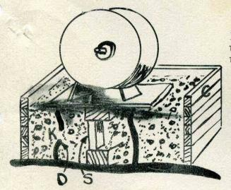
Illustrating how concrete may be used to make a support for a machinery unit.
