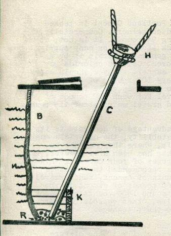
Bulkhead "B" is ruptured at "R". A cofferdam "K" is built around the damaged area. Concrete poured into hopper "H" flows down through chute "C" and fills the cofferdam. It may be necessary to put wedges or pillows into rupture "R" to keep the concrete from walking through the hole, or to restrict the flow of water which would wash out cement. Keep end of tube well down into the laid concrete, as if rupture was small and being filled with tooth paste from a tube.
