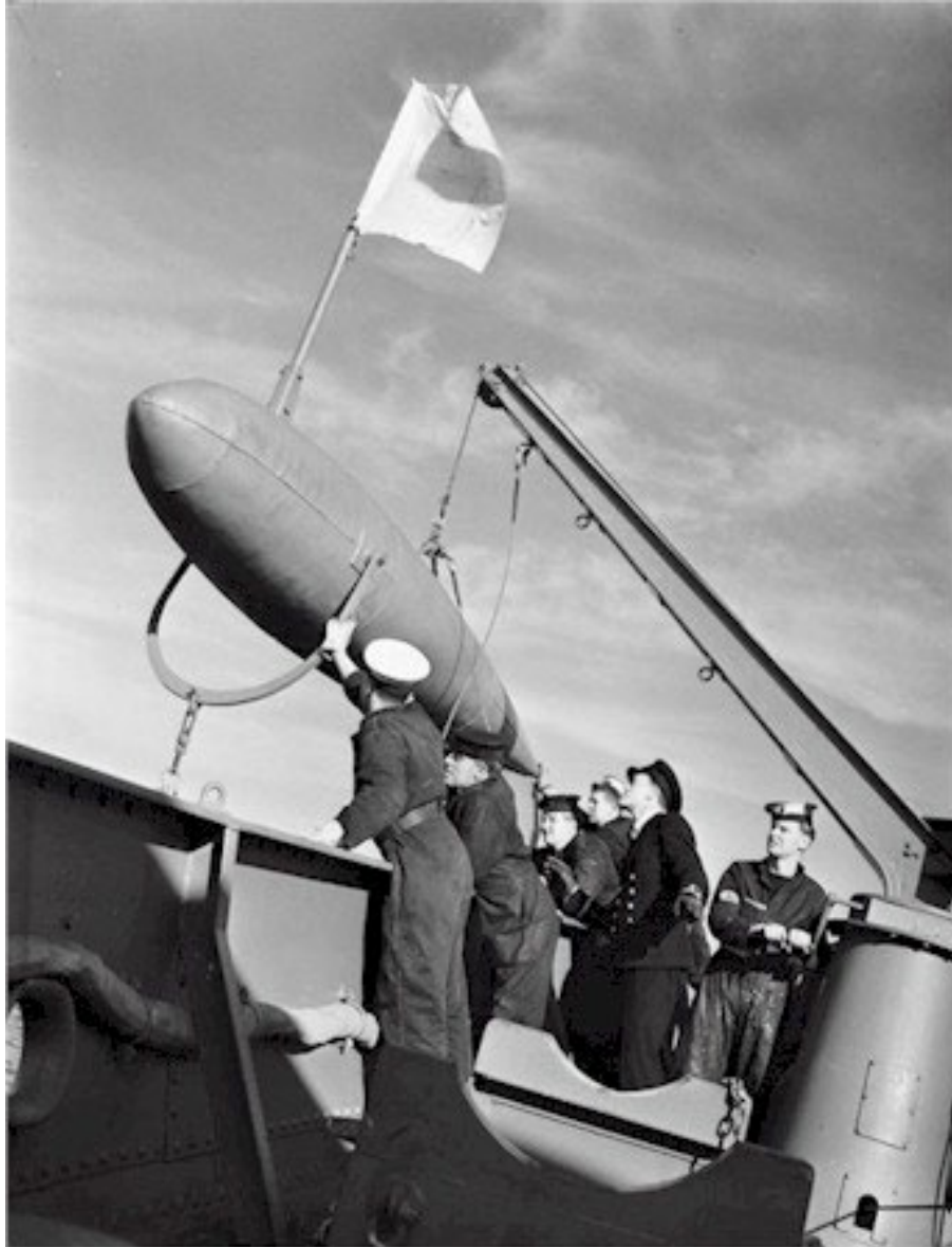
Launching the Oropesa from HMCS Alberni during a training exercise off the coast of British Columbia in March 1941. (Credit: Library and Archives Canada / PA-179942, www.forposterityssake.ca )
