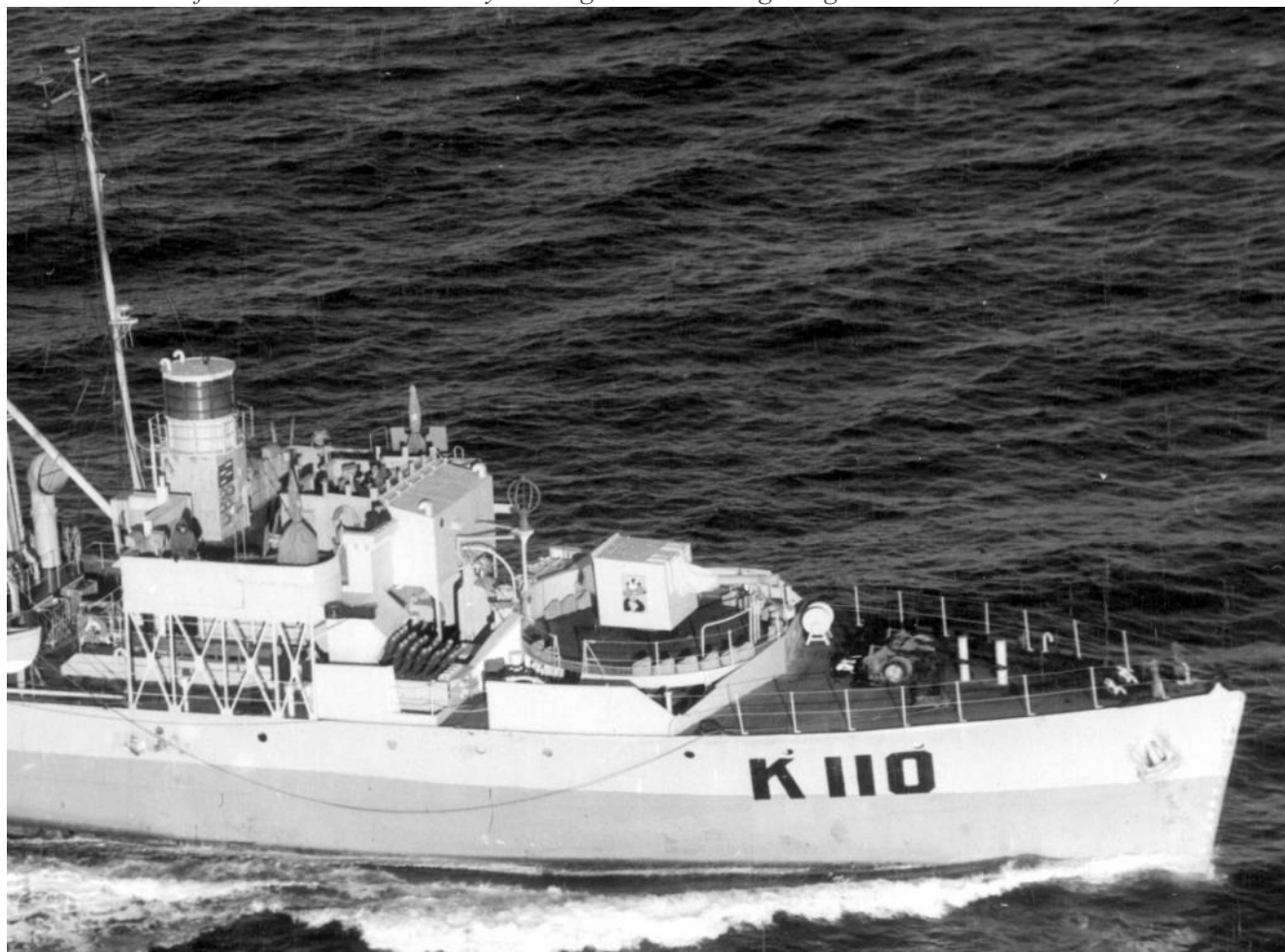
HMCS Shediac. The box-like structure on the front of the bridge is the ASDIC hut. (Credit: Ken Macpherson / Naval Museum of Alberta - Canadian Navy Heritage website. Image Negative Number MC-2935.)
