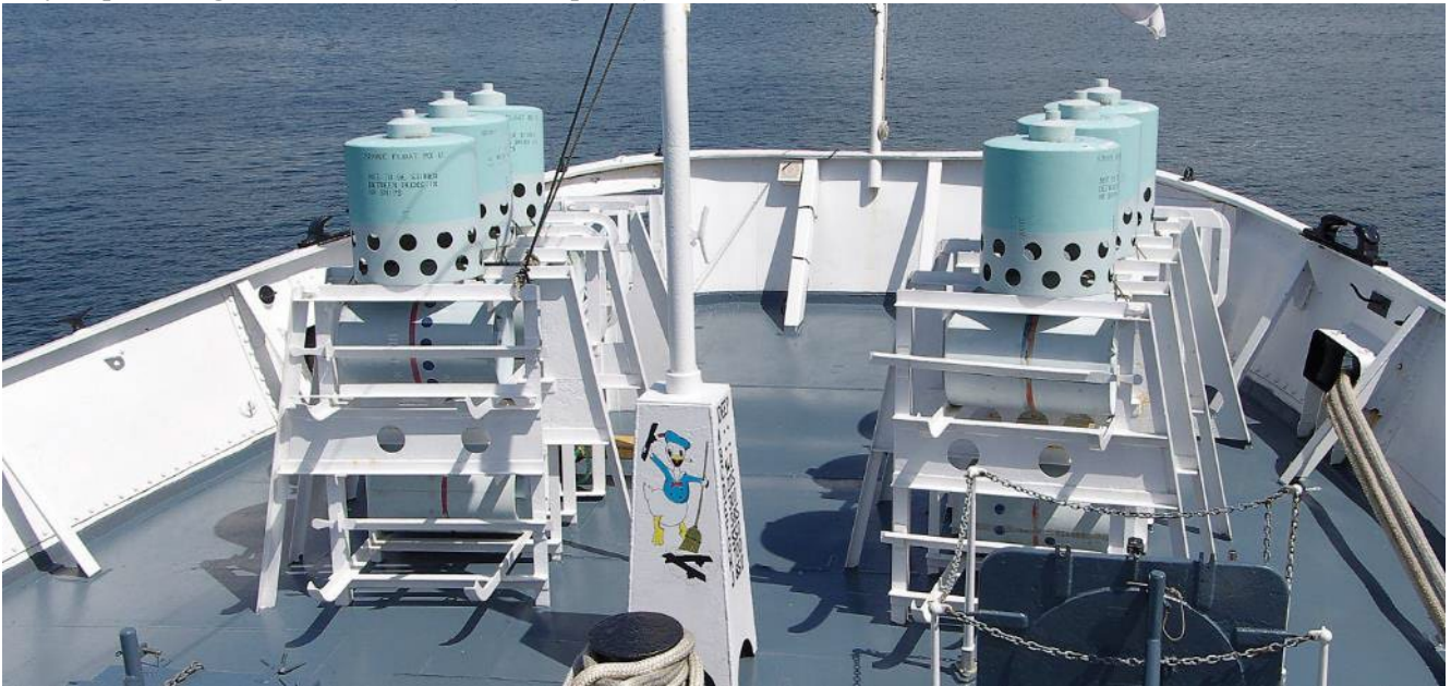
Depth charge launching rails on the stern of HMCS Sackville in Halifax. The small hoist between the rails is used to lift depth charges onto the rails. (author's photo)
