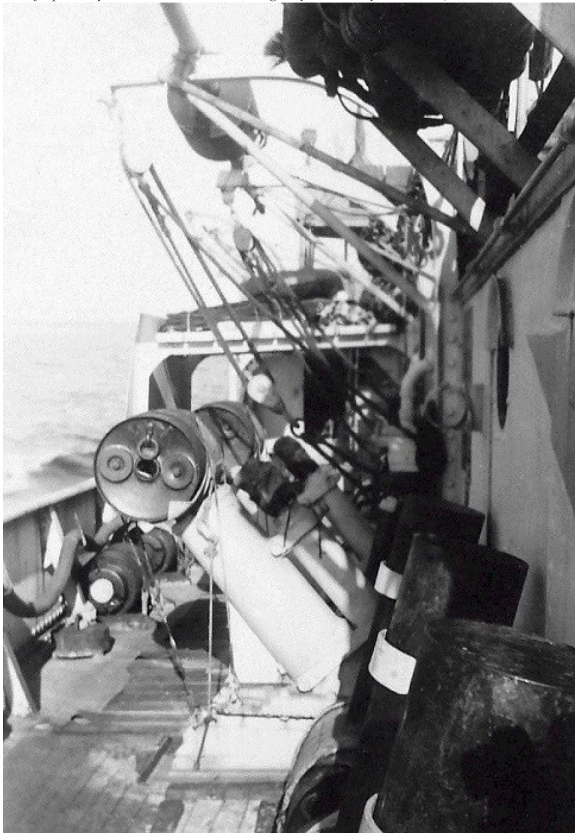
A pair of depth charge throwers aboard HMCS Bittersweet. (Credit: Collection of Ross Maize, www.forposterityssake.ca . Photo has been digitally restored by the author.)
