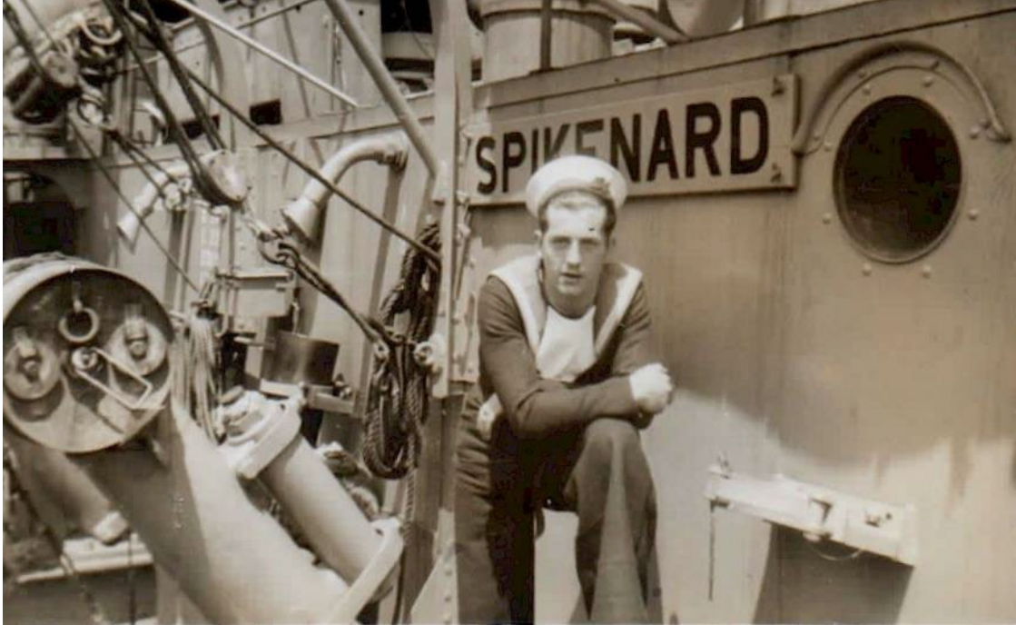
Gerry Zaphe aboard HMCS Spikenard, standing beside one of the depth charge throwers. Two voice pipes can be seen curving out from the bulkhead (wall) behind him, one adjacent to each depth charge thrower. (Credit: Collection of Gerald Zaphe, www.forposterityssake.ca )
