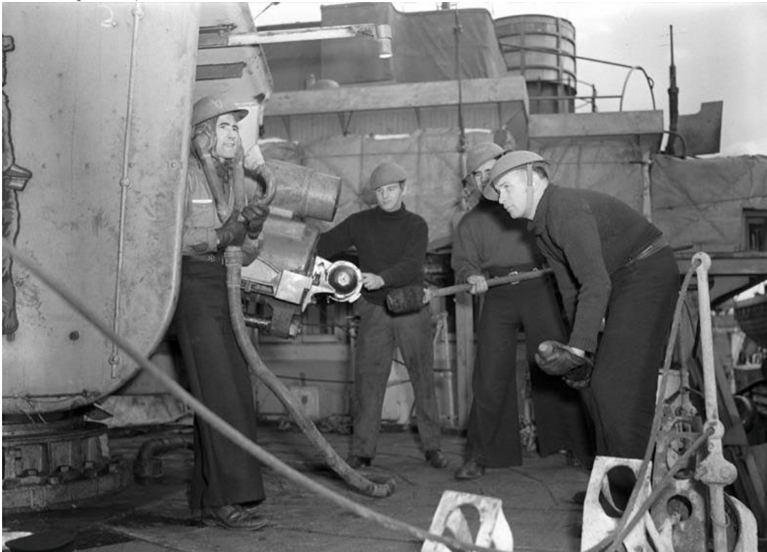
Gun crew aboard HMCS Agassiz, with one of the gunners wearing a flexible voice pipe for two-way communications. (Credit: https://hmcssackville.ca/resources-2/educational-material/photos/ )
