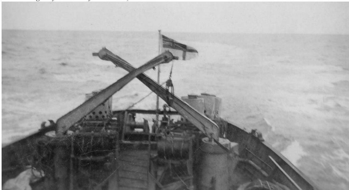
Stern of HMCS Cobalt, showing the two cranes for the minesweeping gear (Credit: Cobalt Mining Museum. Photo has been digitally restored by the author.)
