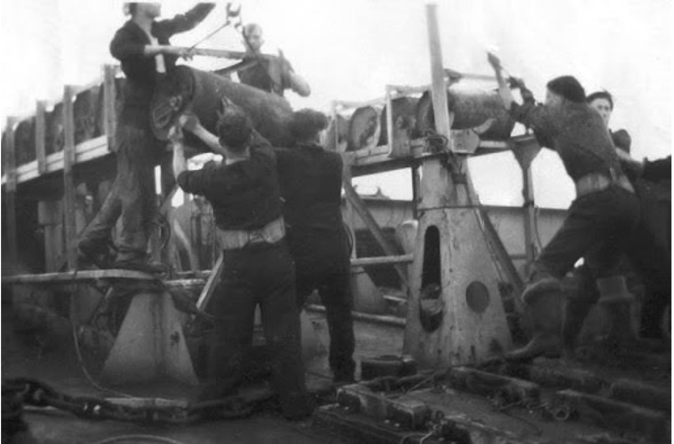
Loading the depth charge rails of the Royal Navy corvette HMS Dianthus. (Credit: http://www.cbrnp.com/RNP/Flower/ARTICLES/Dianthus-1.htm . Photo has been digitally restored by the author.)
