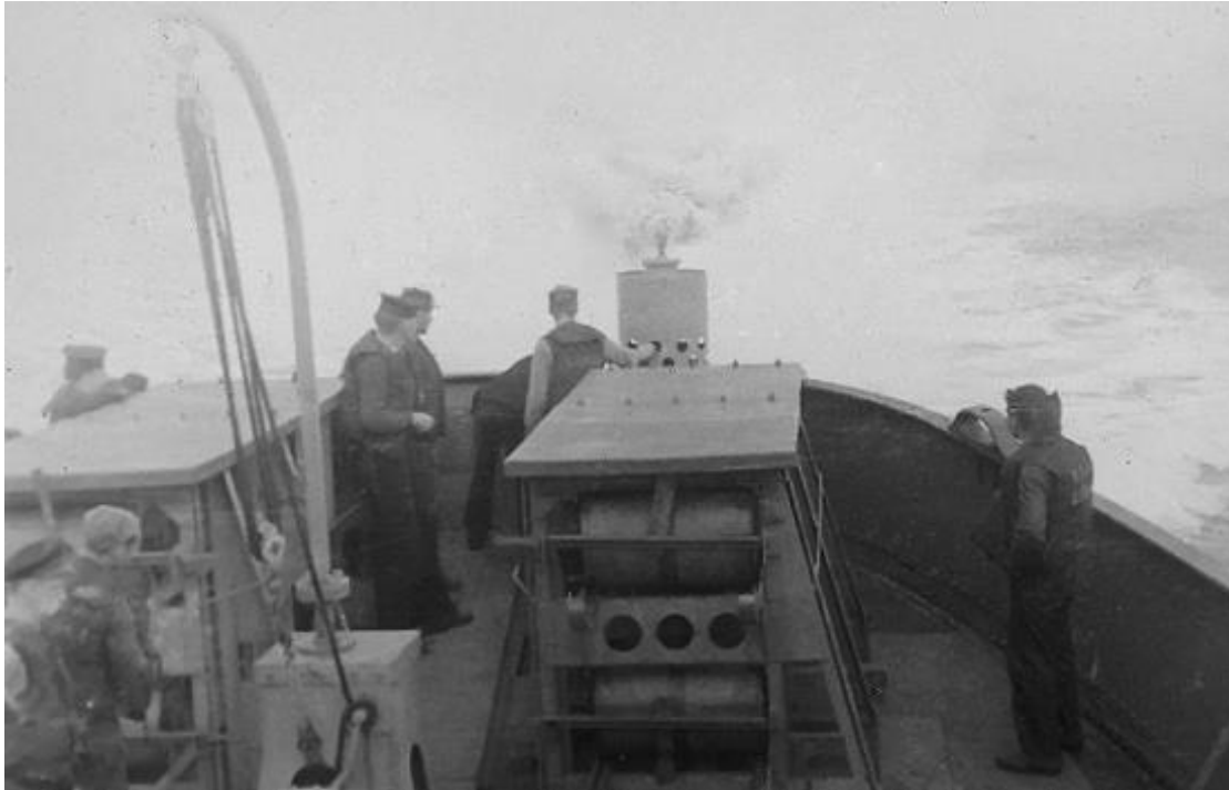
Depth charge rails on the stern of HMCS Lethbridge. The crew are laying a smoke screen using a smoke float. (Credit: Collection of Joseph Roberts, www.forposterityssake.ca. Photo has been digitally restored by the author)
