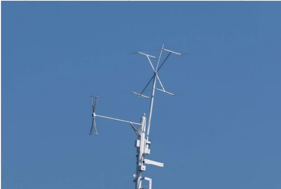
“X” shaped antenna for the SW2C radar atop the mast of HMCS Sackville (author’s photo)
