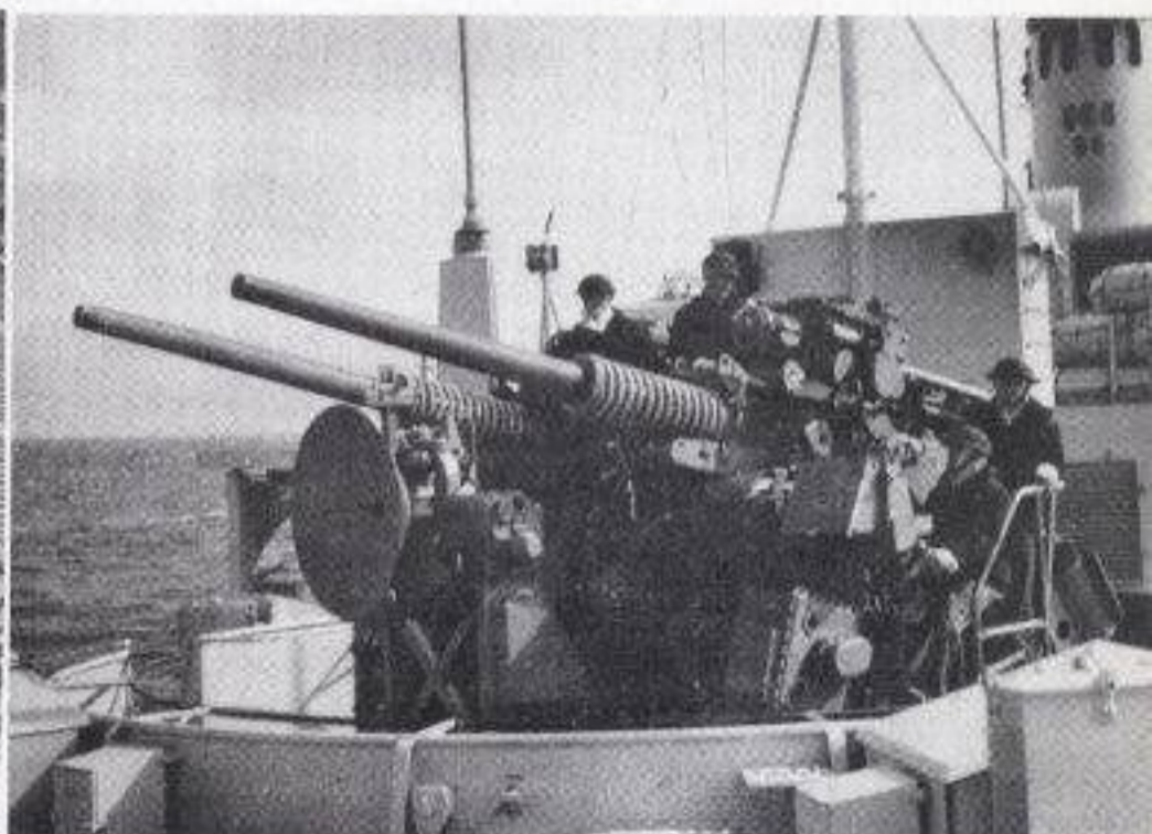
After 3-inch 50 calibre gun with gun's crew closed up during gunnery trials.
