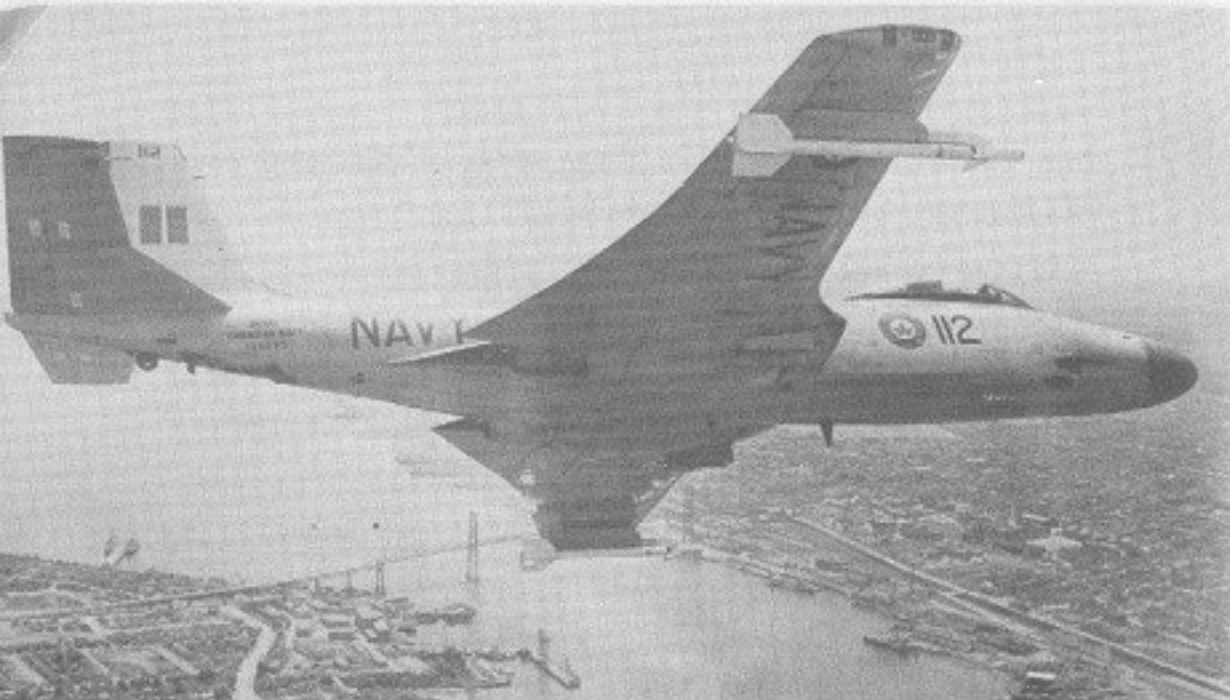
The Navy's fighter aircraft is the twin-jet Banshee armed with Sidewinder air-to-air guided missiles.
