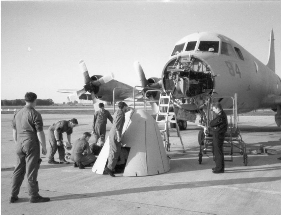
Crew of LC 84 changes out the radome at Rota, Spain On the right, "arms folded," the E8 Killick observes.
