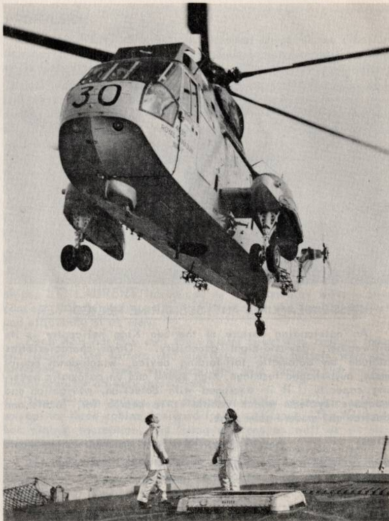
A Sea King helicopter demonstrates the "Beartrap" system for landing helicopters on the flight deck of a Maritime Command helicopter destroyer. The hovering helicopter lowers a thin wire which hauls back a heavier cable from the deck. The slack is taken up and the helicopter begins its descent as the cable is reeled in by the landing control officer on the deck. When the helicopter touches down, steel jaws clamp around the probe to secure the helicopter against any motion caused by rough seas.
